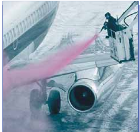
Working from a mobile platform, an airport operative de-ices an aeroplane with 'Ecowing' prior to take-off.
